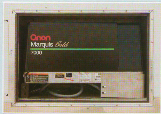
Optional generator can be installed to provide power where electrical hookup is not available.
